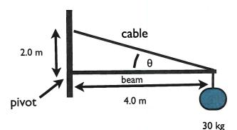
a) [3 pts] Use simple trigonometry to find the angle  $\theta$
